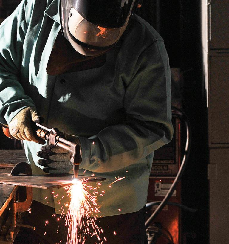
EN 388, the European standard for protective gloves, is recognized globally. The most significant change is the formal inclusion of the ISO 13997 cut test method, with the intent in the future to replace the Coupe test.
