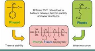
Advanced formulations using siloxane copolymers along with specialized additives enable a wide variety of tailor-made solutions for specific challenge combinations Regulatory mandates, lower engine oil viscosities, and demand for longer engine life and quieter engines are driving growth of AFCs and spurring innovation. Requirements, typically described in terms of load, environment, temperature and speed, result in products that can serve a diverse set of powertrain applications.
