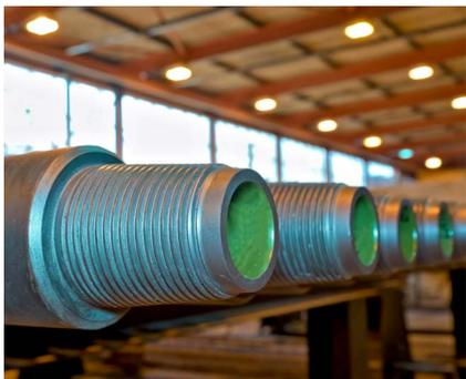
Noble Drilling Corporation had unacceptable failure rates in stainless steel threaded connections on its steerable rotary drilling equipment. Each time the failed drilling sections required removal for repair at a specialty machine shop, the firm incurred extra costs for labor, shipping and refacing the damaged threads; suffered production downtime; and also lost the critical sections for up to a week.
